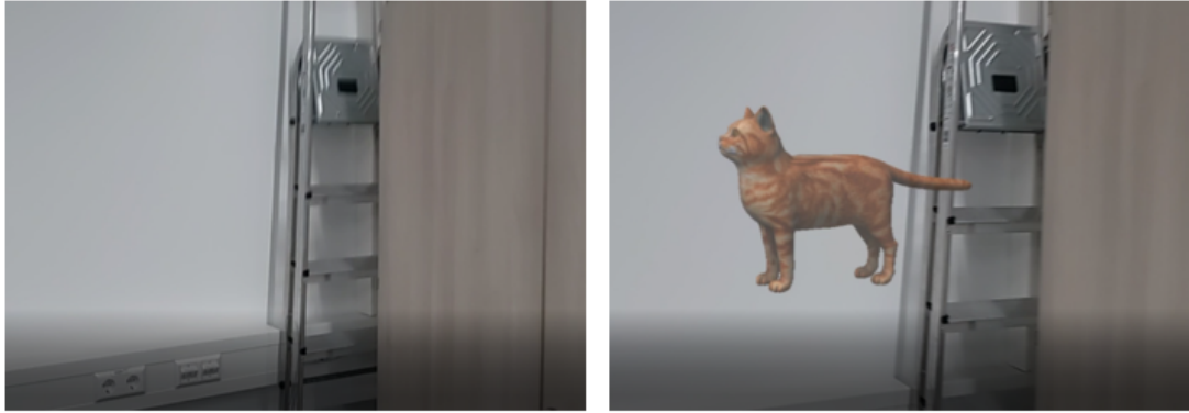
Figure 4.3: On the left image it can be seen that the virtual object is not yet visible. However, as soon as the object was approached to within one meter, it became visible, as can be seen in the right image.
