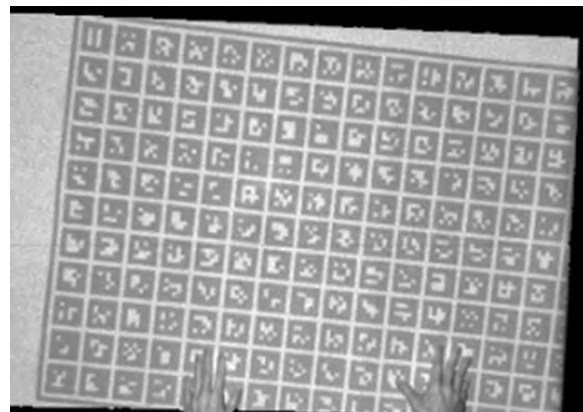
(d) A low cost depth camera is sufficient to get a high contrast image of the markers in the IR-spectrum.
