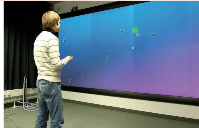
Participant conducting a multi-directional tapping test with a laser pointer device
